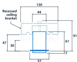
Mounting Arrangement - Plasterboard ceiling
