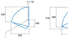
Spot marked for cable entry on both sides. Customer to drill if required.
