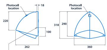
Spot marked for cable entry on both sides. Customer to drill if required.
