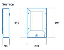
Minimum cut-out - 270 x 420 Maximum cut-out - 600 x 600
